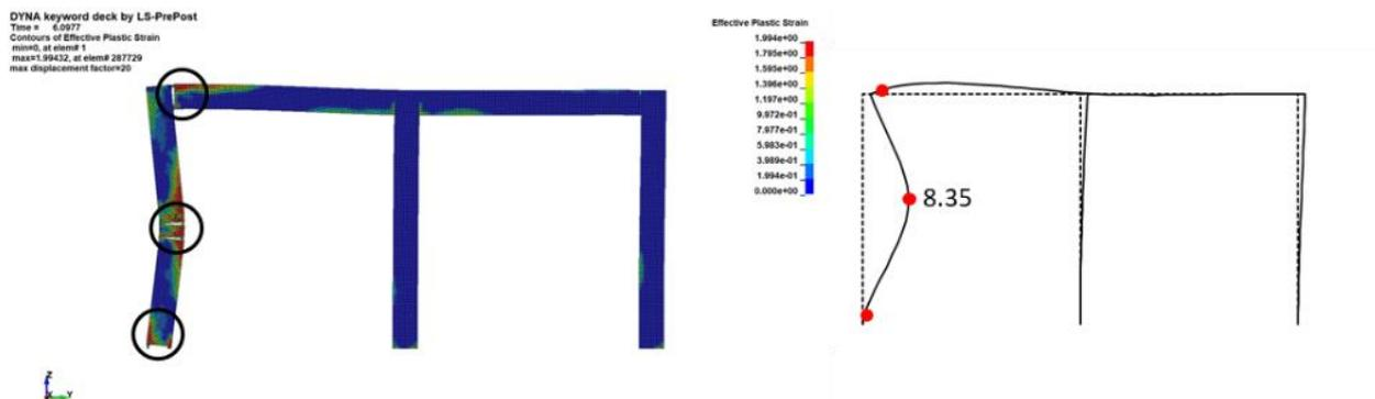
Fig.2 Numerical results of a simple RC frame under blast loading with LS-DYNA and the proposed method
